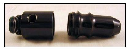
2. Use a adjustable wrench (or a 3/8<sup>th</sup> inch socket) to remove the Regulator Pin Retainer.
