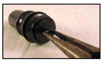
You can also take the Velocity Adjustment Screw out of the bottom and push the piston out with a longer Allen key.
